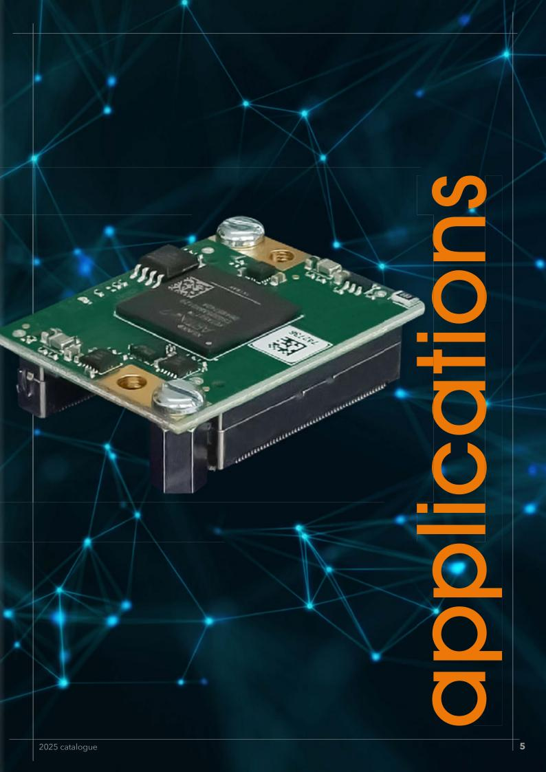
The Ndigo6G-12 is a hybrid ADC/TDC solution for the acquisition of short pulses. It builds on the established platform of the Ndigo5G-10, but takes it to the next level in both, performance and flexibility.
