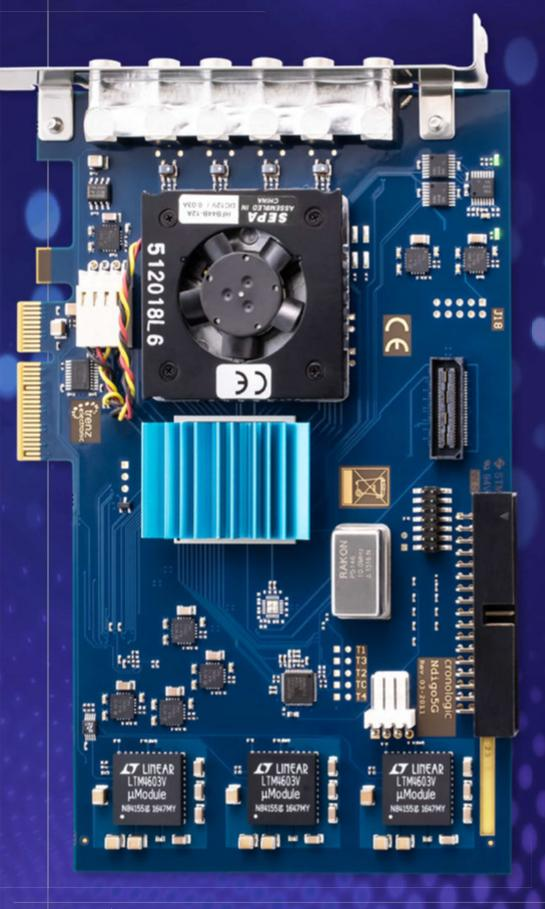
The xHPTDC8 is our most versatile TDC. This is the ideal time-to-digital converter for an infinite stream of time stamps.
