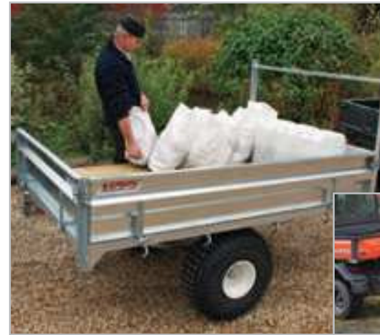
STT400 trailer 1500 x 1000 x 380mm with STT103 tailgate.
