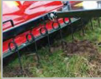
MSP120WT fitted with tine bar, seen here (right) breaking up 'rained in' horse droppings.
