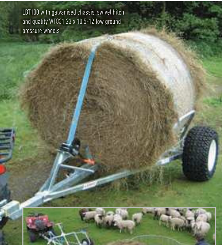
Back up to bale, secure strap
