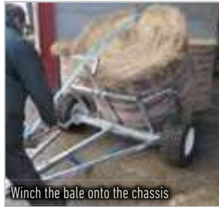
Back up to bale, secure strap
