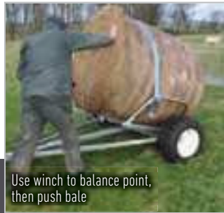
Winch the bale onto the chassis
