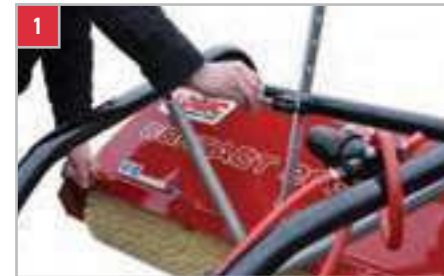
Height adjustment is spring-assisted to allow the machine to be quickly and easily set to the correct working height
