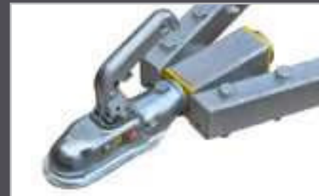
Swivel hitch - bolt-on, to permit fitting in one of 3 positions to match the towing vehicle.
