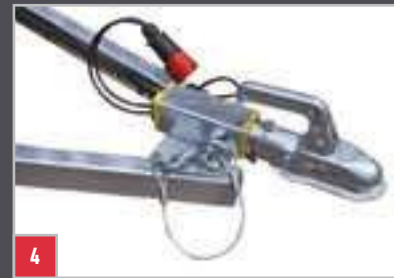
4 Attachment to the towing vehicle features a high quality coupling, heavy duty restraining cable, 7 or 13 pin electrical plug with storage socket and drawbar skid.
