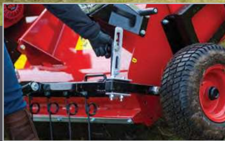
The optional MSP121 tine bar is easily fitted and adjusted to contact more solid heaps of rubbish or animal droppings, breaking them up before the brush. It is easily adjusted by turning the large hand screw (above) to release and reposition the bar stem into one of 3 secure locating slots.
