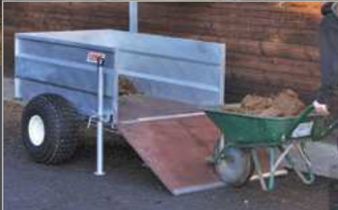
TST400 tipping trailer 1500 x 1000 x 500mm tapered body with lower sides for easy access. Features include a tailgate which can double as a loading ramp. Options include a RT710-01 jockey wheel and RT710-02 prop stands.
