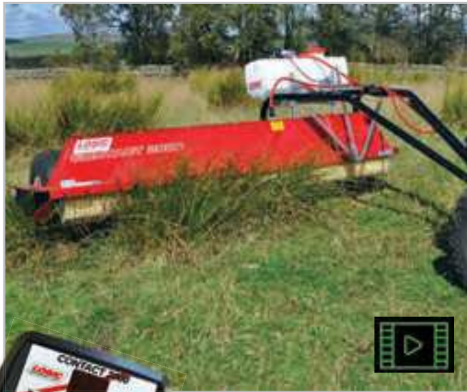
CTM600W Grassland model, 6.0 metre working width as used to treat the before/after field above.
