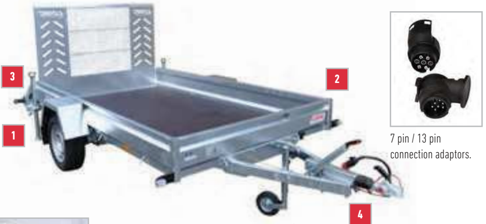
2 Monoque construction with 'A' frame drawbar, Al-Ko suspension, one piece axle (1300kg) featuring rubber progressive action with excellent dampening. All protected with hot dipped galvanising for long life.
