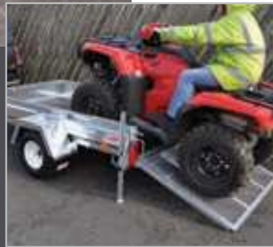
XRT610E with 20.5x8-10 wheels and tyres with optional XT106 mesh ramp tailgate and RT710-02 rear prop stands. Ideal for transporting an ATV or garden tractor.
