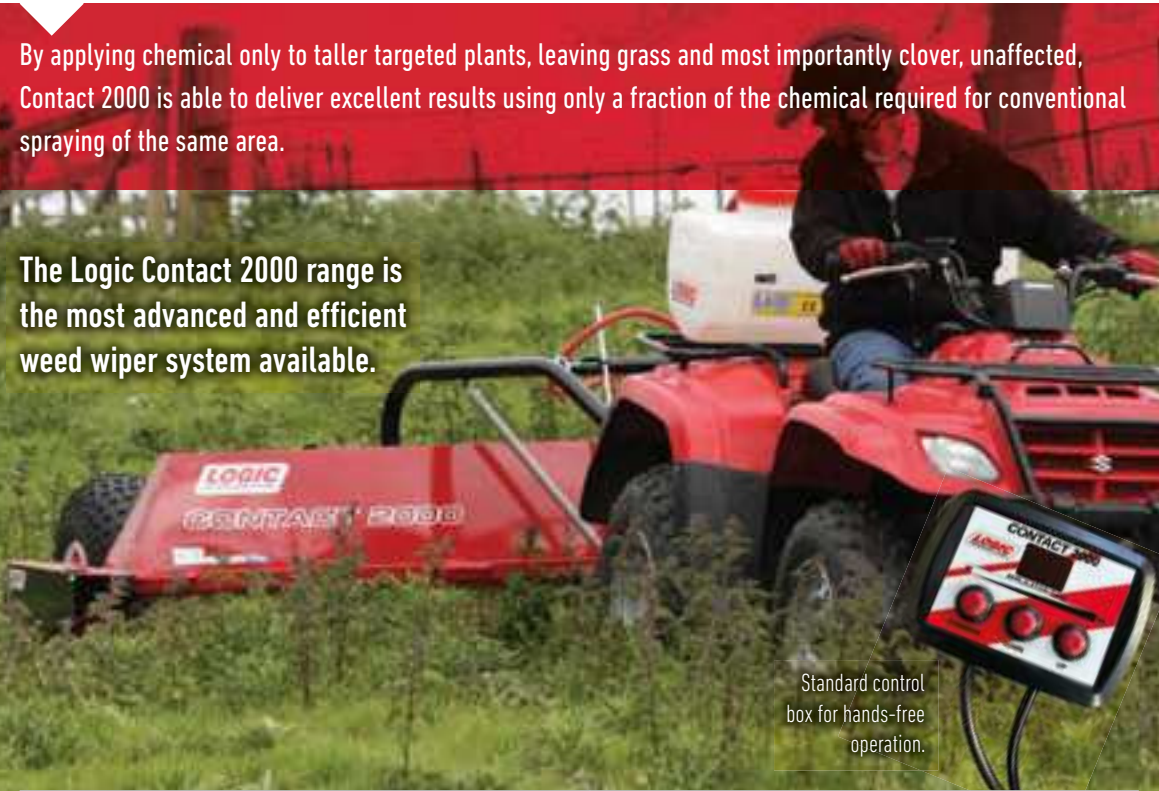
Height adjustment is spring-assisted to allow the machine to be quickly and easily set to the correct working height
