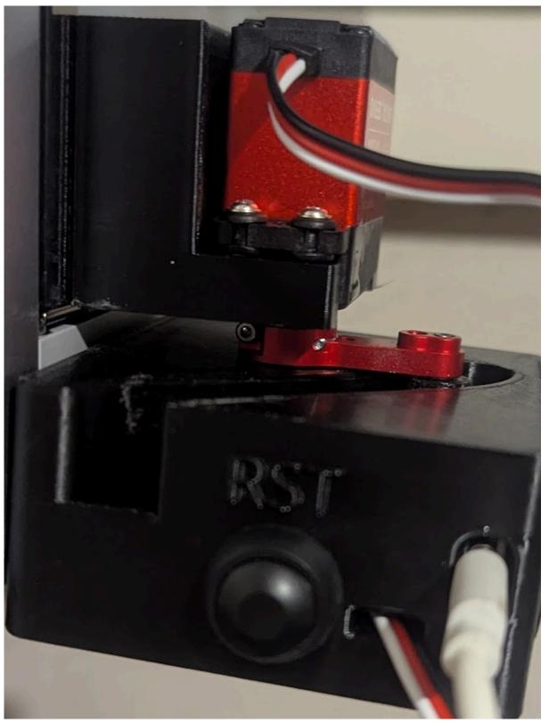
Now by default the servo should be in a closed position. If you can't assemble it due to the servo position, refer to the following chapter on calibration.
