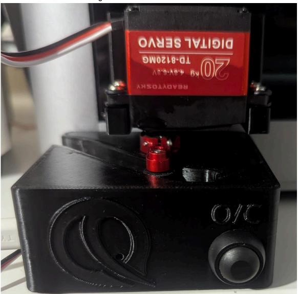
Once that is in place, you can add the servo with the pointy screws supplied. Ensure the servo is held tightly, but not more.
