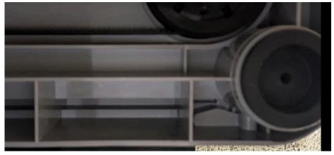
All you need to do is lift your bambu, or pull it over the edge of a shelf like I did for this picture. Then push the rail part in like this (looking from below):
