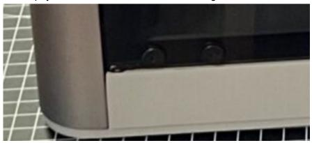
Don't worry, your door will not move as it's still held by the upper hinge. Then attach the servo holder with the two provided M3 bolts in order to have it positioned like shown below. Be careful to not overtighten the bolts.
