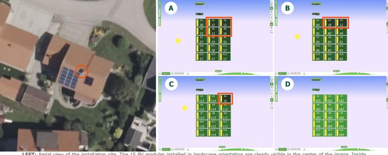
**LEFT:** Aerial view of the installation site. The 15 PV modules installed in landscape orientation are clearly visible in the center of the image. Inside the red circle, the chimney that casts its shadow on 4 modules during the morning hours.
