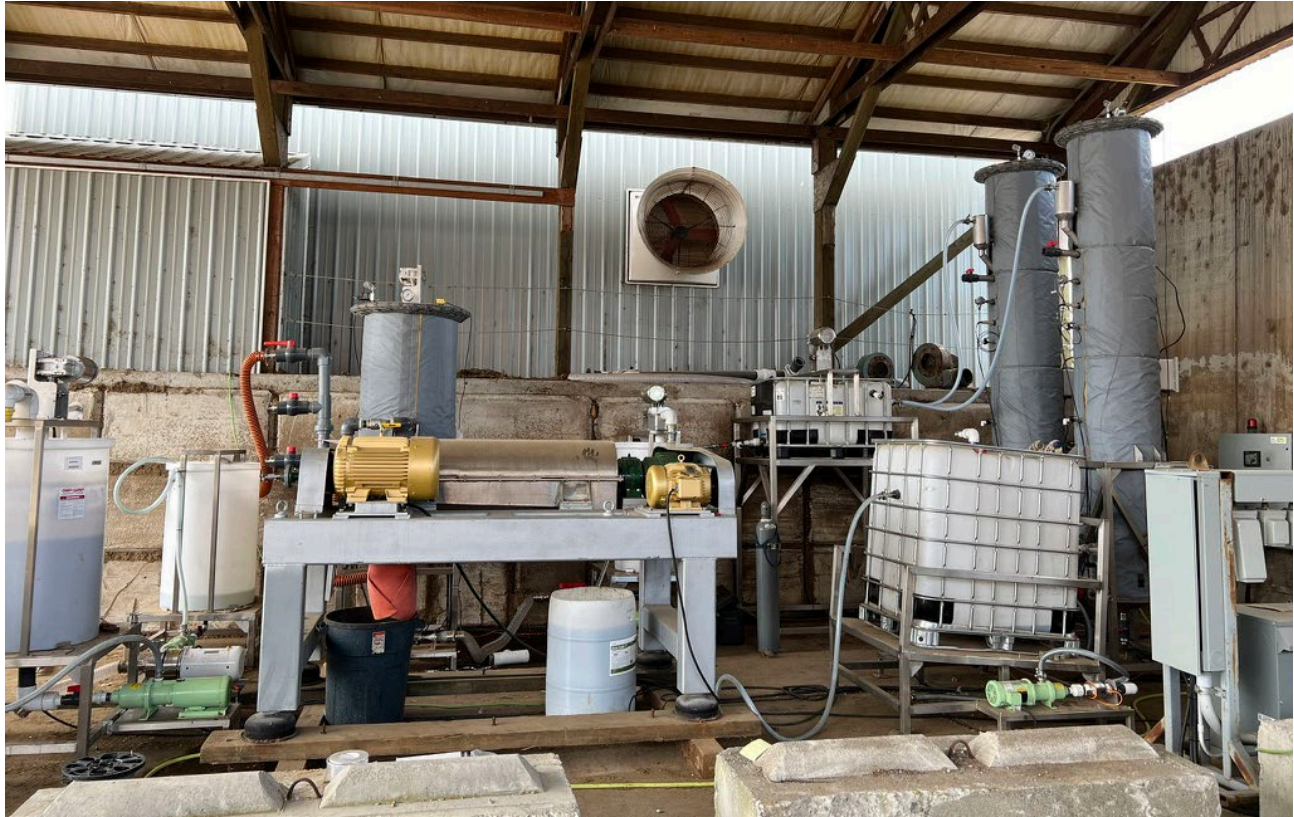
Figure 2. The pilot-scale Intensified Versatile Anaerobic Digestion (IVAD) system
