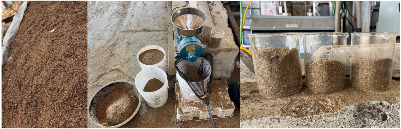
Figure 3. Size reduction process by grinder and the ground solids
