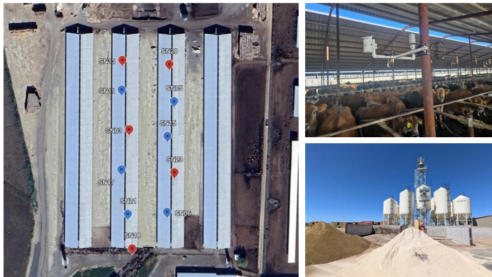
Figure 11: Free stall barns at Royal Dairy Farm with GHG sensor nodes and an automated commodity and mixing TMR station under construction to accurately dose the additive Bovaer® (3-nitrooxypropanol, 3-NOP) for pen studies.
