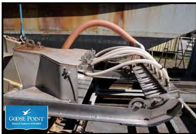
Figure 5. Prototype precision harvest head, which uses water jets to float oysters onto a conveyor belt (image via Goose Point Oysters).
