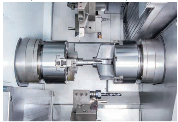
Twin spindles simultaneous part catching
