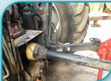
P.T.O. with chains fitted
