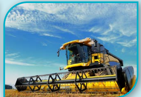
The header on a combine is powered with a P.T.O.
