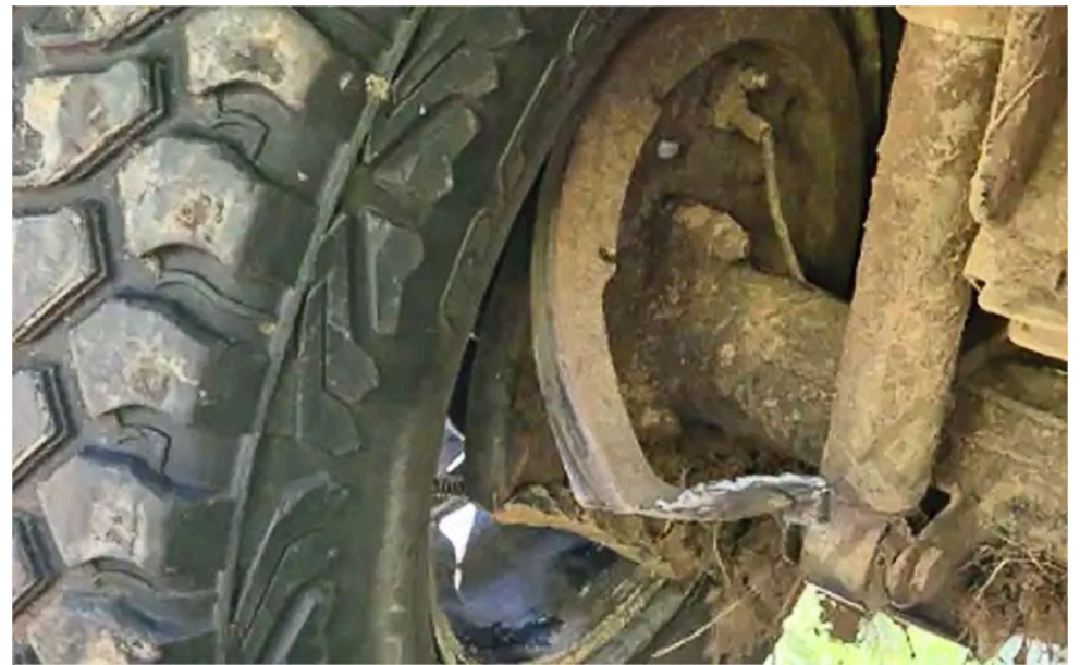
Left-hand rear wheel showing damage to the underside and evidence of metal components being subjected to high temperature. Photo: Fire and Emergency / supplied
