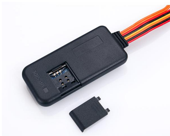
Figura 1. Socket sim card SKT119
