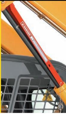
The lift arm is raised by two NitroSteel<sup>®</sup> cylinders. Lift arm support device is provided.
