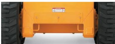
Tie-downs located at the front and rear of the machine make for secure over-the-road transportation.
