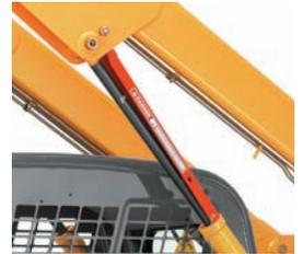
Service safety — lift arm support device locks the lift arm in the raised position during maintenance and service.
