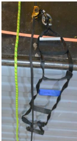
Setup – Green: Belay/Safety – Black Main
