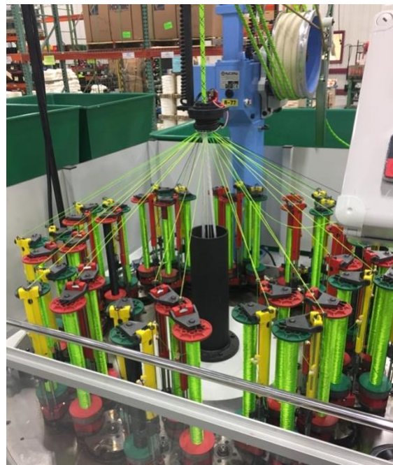
Each bobbin is a yarn that is being braided around the core of the rope to form a sheath.
