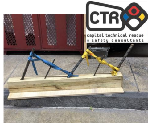
Picket Anchor System Examples 3 Picket System in 1 - 1 - 1 Configuration ~1,800 lbs Rating
