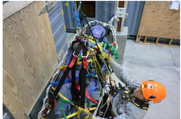
Horizontal Litter with Litter Attendant using a SOFs and a Prusik Safety
