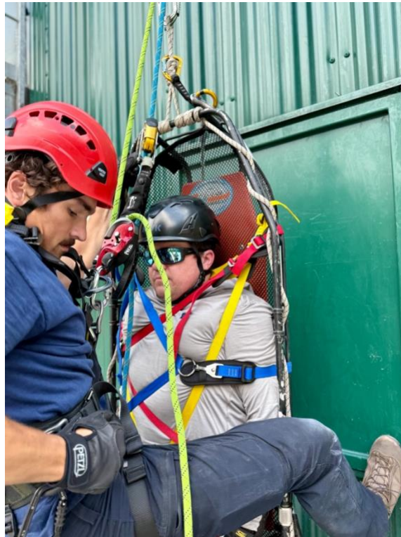
Patient tied into litter with CMC Patient Tie In System and directly connected to the litter with the Pelvic Attachment Strap (yellow). Attendant on “Long Tails” from the MAP (Master Attachment Point). If the victim is in a low angle scenario or anywhere that their head maybe lower than their feet, they should have a second Pelvic Attachment Strap keeping tension towards their feet so they can’t slide upwards.
