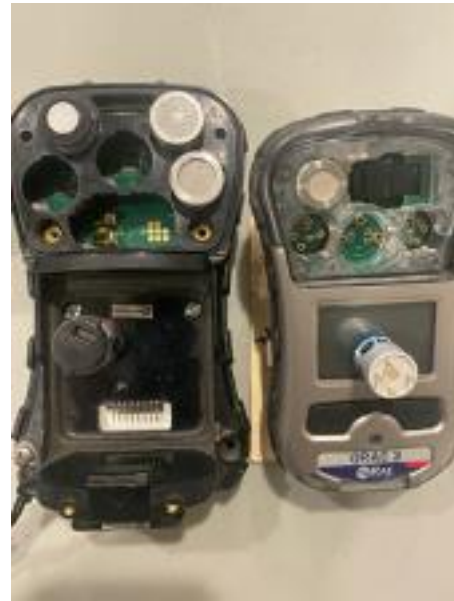
Internal view of sensors in a MultiRAE and QRAE 3 Meter. Two sensors are turned over to show the different electrical connections.
