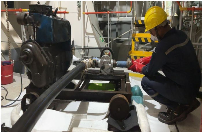
Deploying oil transfer engine pumps on a vessel to transfer oil from damaged tank to tankers directly
