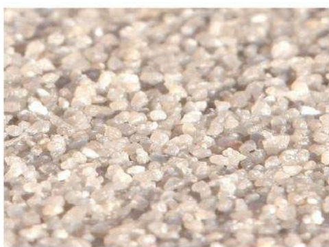
Fig. 2: Quartz sand (above) is reduced with graphite in smelting reduction furnace (schematically, right) to raw silicon.
