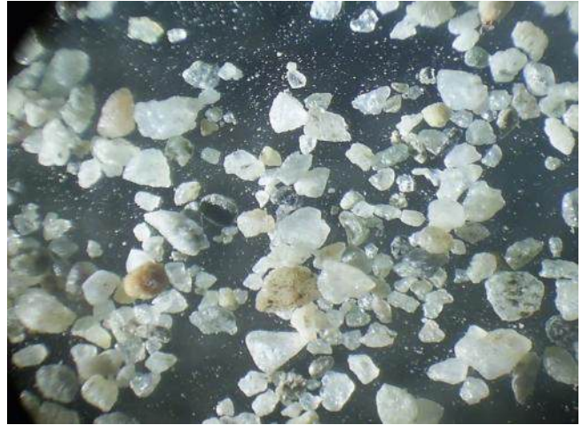
Fig. B – Crust impurities removed by attritioning
