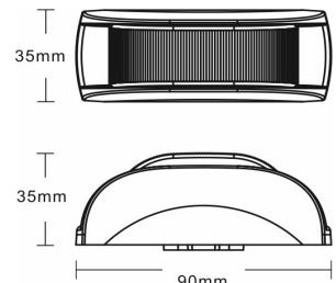
**F1203200:** 3.5" BLUE FLASHING WARNING LIGHT, 180 DEGREE HORIZOMTAL VIEW, 19 FLASHING PATTERNS WITH SIMULTANNEOUS OR ALTERNATING, SAE J845 CLASS 1. BRACKET (INCLUDED) MOUNTING.
