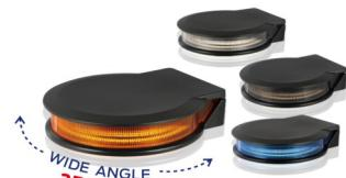
**F4004200:** 4" RND BLUE FLASHING WARNING LIGHT, 270 DEGREE HORIZOMTAL VIEW ANGLE, 19 FLASHING PATTERNS WITH SIMULTANNEOUS OR ALTERNATING, SAE J845 CLASS 1. BRACKET (INCLUDED) MOUNTING.
