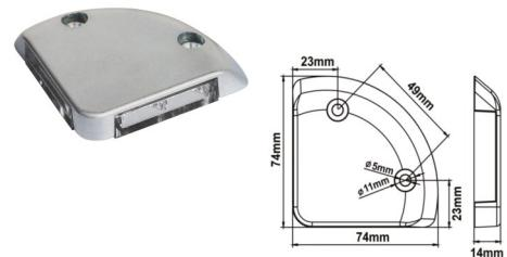
**F0403505:** 3" WHITE, CONER BOLTS MOUNTING, ZINC-ALLOY CASTING HOUSING WITH PC LENS, 6 FLASH PATTERNS WITH SYNC FUNCTION. TAIL LIFT SAFETY LIGHT, 12-36 VDC
