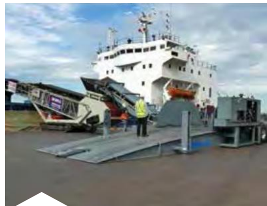
Truck unloaders and track-mounted conveyors
