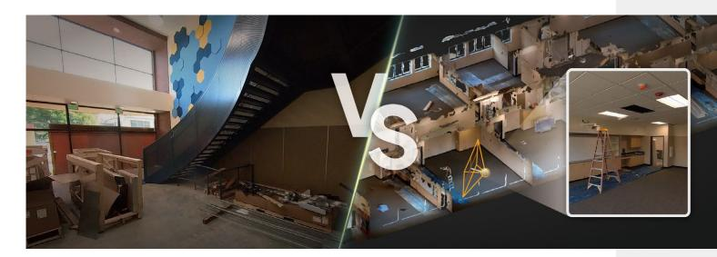
360 photo documentation is a popular technique involving the use of consumer-grade 360 cameras for capturing panoramic photos or videos to create a virtual tour of a site. This easy-to-use method, widely adopted by busy engineers onsite, brings a novel way of recording existing as-built site conditions for visual progress sharing or evidence collection for potential future disputes. Vendors like Insta360 and Ricoh offer some easy to use and affordable hardware to collect his type of data.
