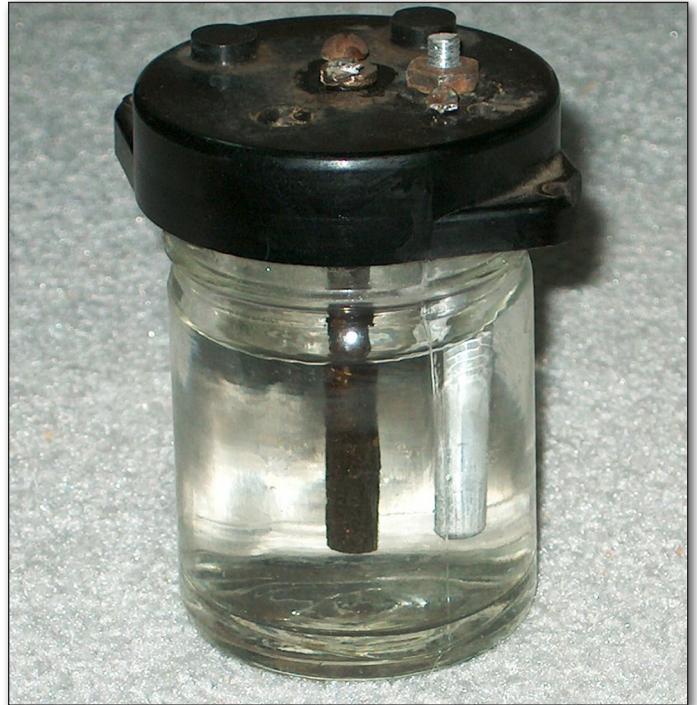
Two Of These Electrolytic Rectifiers. Dump The Electrolyte And Replace When The Speaker Volume Goes Low
