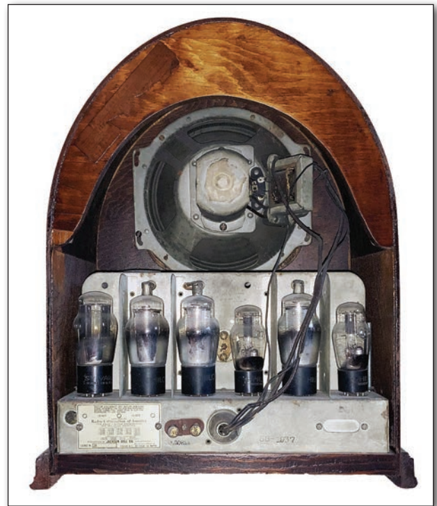
Rear View of Model 88, Version 1 Used rectangular I.F. cans and very similar chassis metal to that used by Flint
