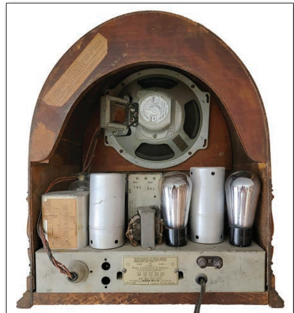
Model 89 Rear View Note the square I.F. cans and rear speaker plug
