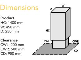
Height HC is combination of Height base frame 340 mm Height DC outlet 1060 mm
