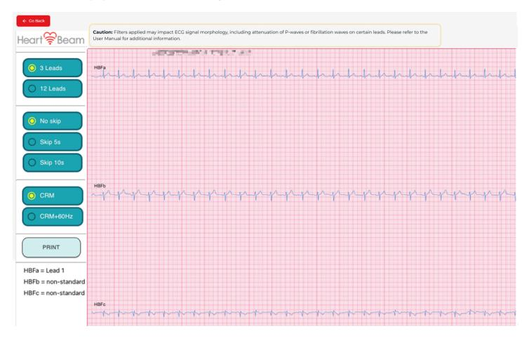
**NOTE:** The CRM Filter is applied to all recordings. The CRM filter includes methods to reduce Electromyographic (EMG) and Baseline Wander noise. These filters cannot be disabled by the user. For a description of these filters see Appendix A.
