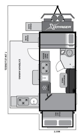
SIZE CLOSED - INCLUDES A/C Length 7.2m - Width 2.35m - Height 2.75m
