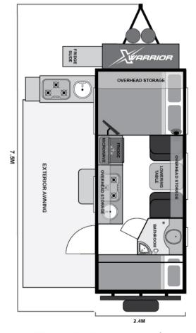
SIZE CLOSED - INCLUDES A/C Length 7.5m - Width 2.4m - Height 3.1m
