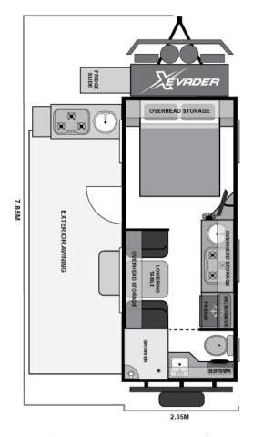
SIZE CLOSED - INCLUDES A/C Length 7.85m - Width 2.35m - Height 3.1m
