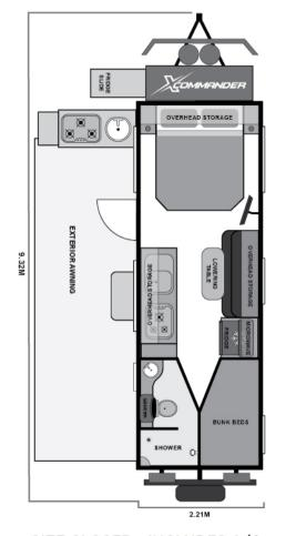
SIZE CLOSED - INCLUDES A/C Length 9.32m - Width 2.21m - Height 3.1m
