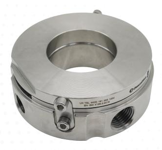
We design our holders for raised face flanges as standard. Options such as RTJ or tongue-and-groove designs are available on request. The additional option of a PFA or Tantaline coating protects the holders in corrosive environments.
