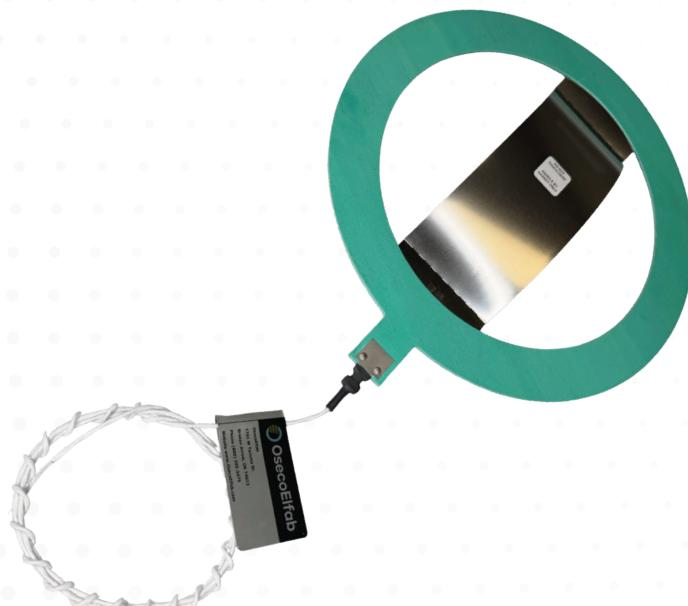
Our CMS (Crowned Metal Sensor) is used with larger rupture disks, where the disk crown may extend beyond its holder and interfere with standard flat sensors.
