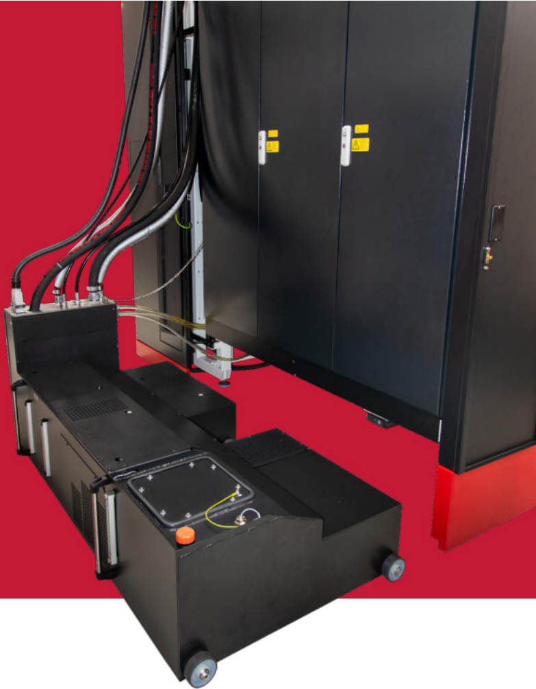
Hybrid Cabinet The fully integrated hybrid unit which supplies the enhanced Kern temperature management provides the best machining quality – and only requires a small footprint.
