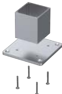
160 x 160mm Screw on flanged base (90 x 90mm post) (130mm Hole centres) Code: FP9020xx
