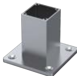
120 x 120mm Welded flanged base (60 x 60mm post) (89mm Hole centres) Code: FPPC6020
