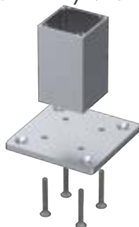
120 x 120mm Screw on flanged base (60 x 60mm post) (89mm Hole centres) Code: FP6020xx
