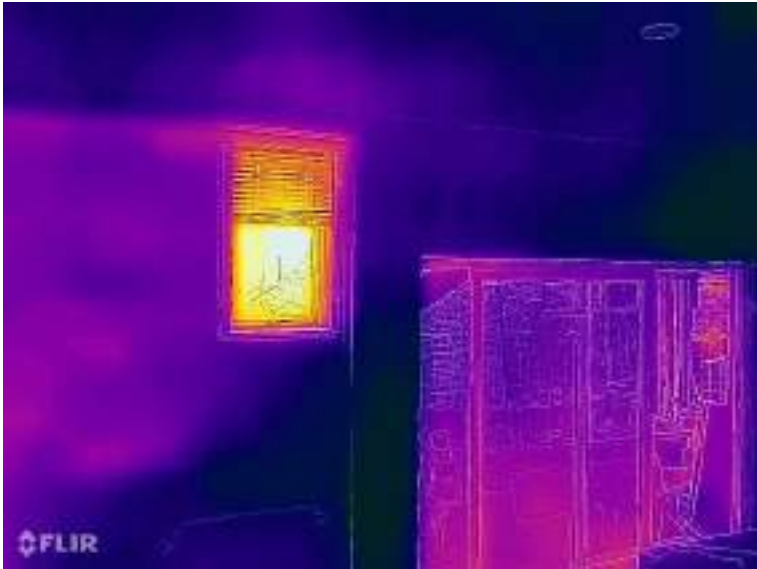
Thermal imaging of the external walls shows insulation between the concrete structural members
