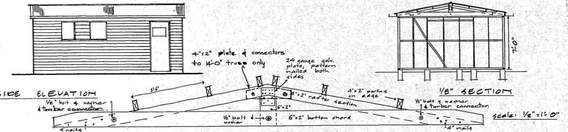
Truss as used for 14'0" span placed directly over stud at 8'0" & 6'0" c/s. to suit length of building
