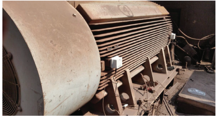
SWI - Eneritics sensors installed on Drive End and Non-Drive End of a Motor application
