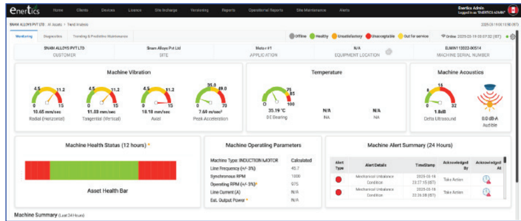
SWI – EnerTics Cloud Dashboard with real-time sensor data, analytics and alarms.
