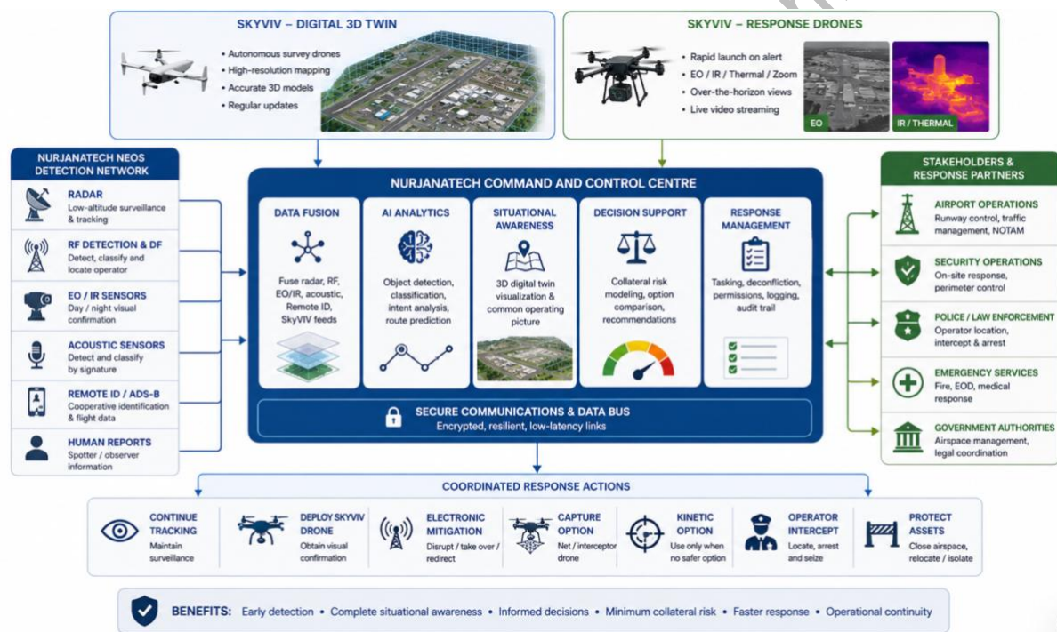
Figure 4: Integrated operational solution. From detection to decision: a connected system for complete situational awareness and coordinated response
