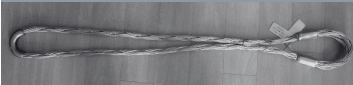
The same Strop untied from the knot. Note the minimal set remaining in the cable.
