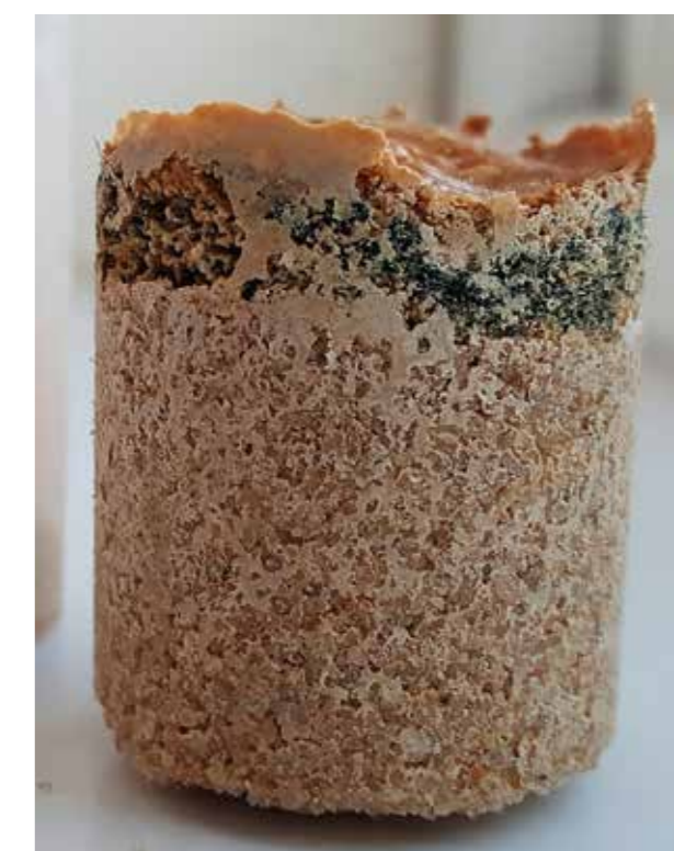
▲ Figure 2. A sand column bound by microbially induced calcite. (© Dr Ismael Justo-Reinoso)
