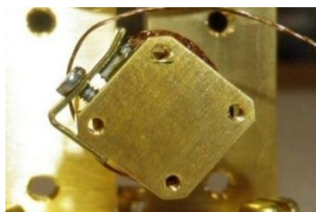
Step 3a: Thermometer clamped to the mounting surface
