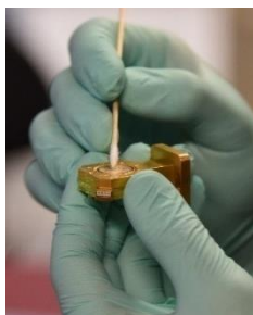
Step 1: Clean surface & apply grease
