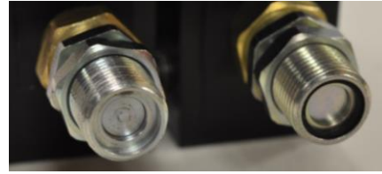
Fitting missing O-ring (left) and with proper O-ring (right)
