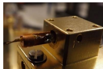
Step 3c: Thermometer installed in the plug
