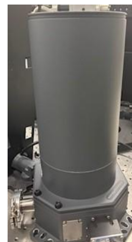
Step 10: Upper vacuum housing installed.
