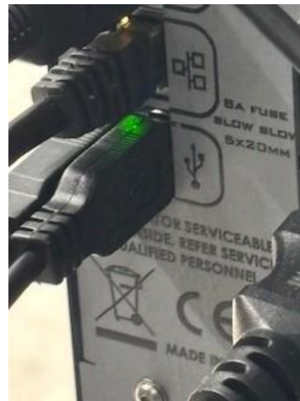
Step 11b: Connecting the Temperature Controller to the System Control Module (back of System Control Module).
