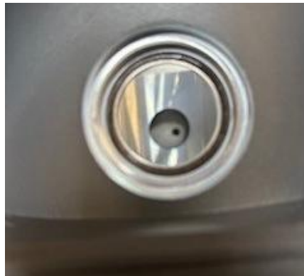
Step 5: Window centered on O-ring.
