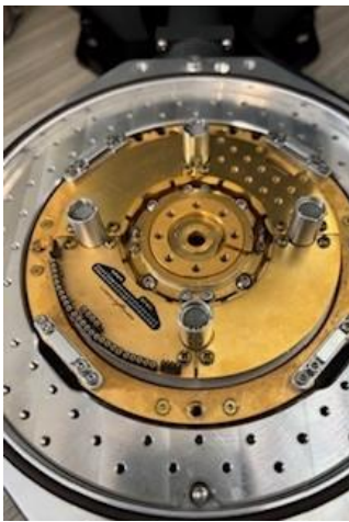
Step 1: Bare sample chamber (sample chamber surround plate installed).
