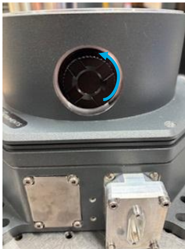
Window cover installed on standard vacuum housing.
