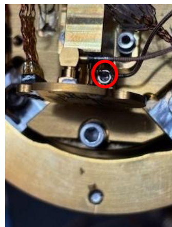
Step 5: Sample mount exchange, set screw circled in red.
