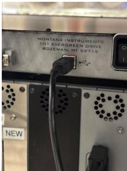
Step 11b: Connecting the Temperature Controller to the System Control Module (back of Temperature Controller).
