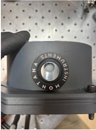
Steps 1-2: Using window tool to unscrew the retaining ring.
