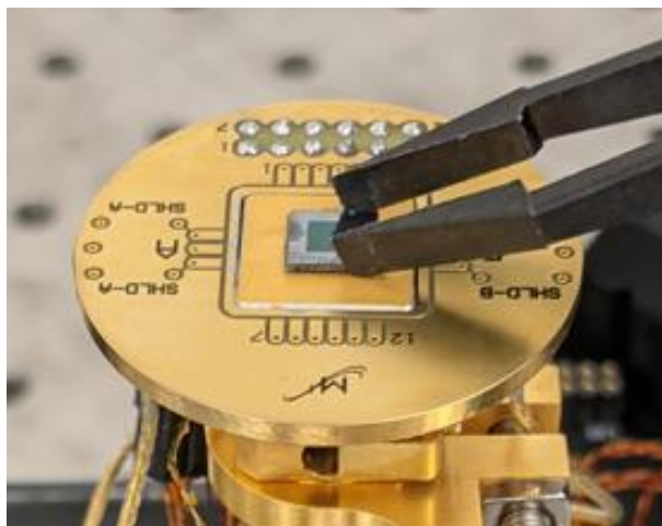
Step 3: Attaching new sample.
