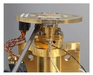
Attach sample mount to exchange boss
