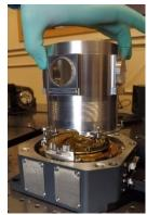
Step 4: Lifting off the radiation shield assembly
