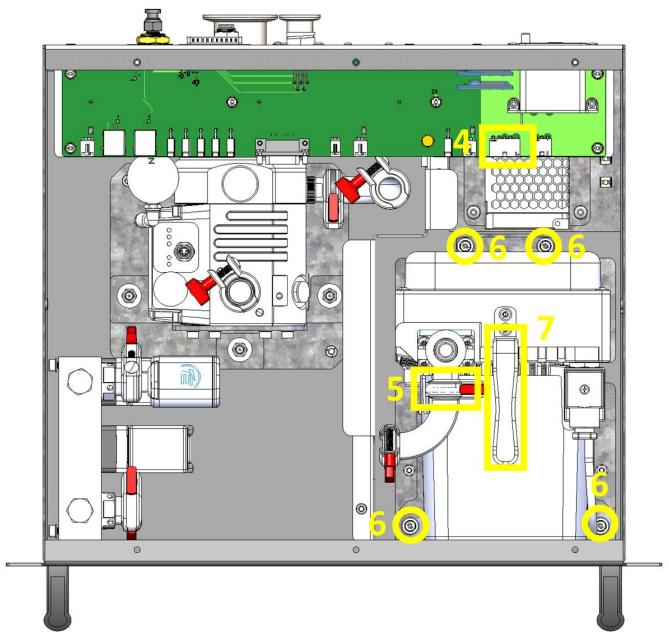
7. Carefully lift the mXD3s by handle to remove from Vacuum Control Unit to perform maintenance per the Edwards mXD3s manual.
