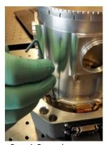
Step 4: Removing screws
