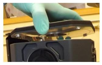
Step 1: Lifting off the lid with protruding bosses on the underside
