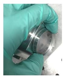
Step 1: Unscrewing threaded tension ring
