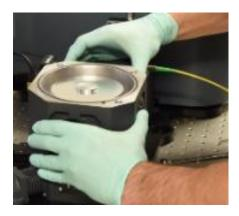
Step 2: Lifting off the window assembly
