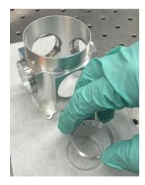
Pressing tension ring onto the window
