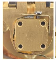
Step 3a: Thermometer clamped to the mounting surface
