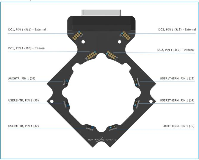
CryoAdvance-50 PCB diagram
