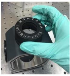
Steps 1-2: Using the window tool to unscrew the retaining ring
