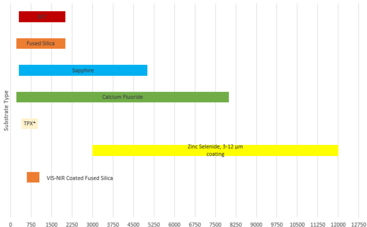
Figure 4: Selection of window substrates and where their transmission ranges fall within the electromagnetic spectrum.
