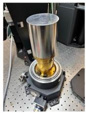
Step 2: Lifting off the 40K radiation shield.
