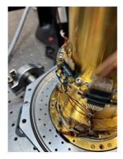
Step 3: Disconnect installed RF lines from sorption cooler assembly.
