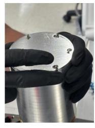
Step 11: Installing the sorption cooler assembly lid.
