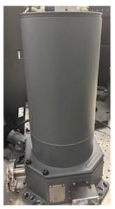
Step 13: Upper vacuum housing installed.
