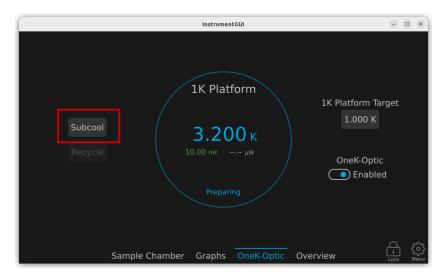
**Recycle-** Brings system back to stabilizing state, can be done if liquid helium remains in the system or not. Note that there is a lockout period when the system is actively subcooling where Recycle cannot be engaged. It begins automatically if no liquid helium remains.
