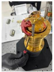
Step 4: Removing the pin shipping bracket.
