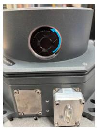
Window cover installed on standard vacuum housing.
