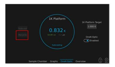
The Recycle process, once started, cannot be stopped. The Subcool button cannot be engaged again until Recycle is complete and the system enters the Stable state. During Recycle, the 4K and 1K platforms will warm up slightly. The chamber will still be under vacuum and under 5K during this time.
