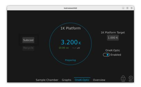
**Subcool-** When the system determines that enough liquid helium has been created and subcooling can begin, the Subcool button will become available to press. Subcooling will only begin on user input. The longer the system is left in the Preparing state, the longer the Subcooling state will be (up to the max of ~8 hours).
