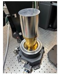
Step 9: Lower vacuum housing installed.
