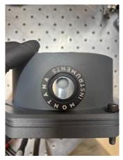
Steps 1-2: Using window tool to unscrew the retaining ring.
