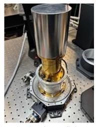
Step 8: 4K lower radiation shield installed.
