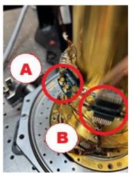
Step 6: Sorption cooler assembly operational wiring (B). RF user wiring (removed)(A).
