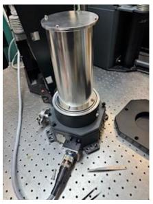
Step 12: 40K upper radiation shield installed.
