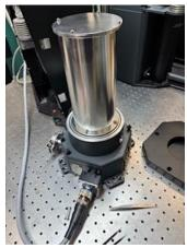
Step 1: Lifting off the uppervacuum housing.
