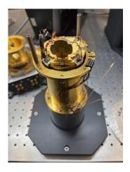
Step 5: Soprtion cooler assembly removed and set in tabletop holder.
