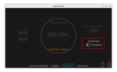
**Dormant -** The OneK-Optic device is above operational temperatures. The system remains in Dormant state until the Cryostation cools to near-base. This encompasses the Pre-Cooling mode.
