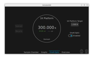
**Stabilizing -** The OneK-Optic device is waiting for internal temperature readings to settle at a range that allows for Helium Desorption mode. The system will enter Stabilizing state from Dormant state automatically when temperatures of the device have dropped low enough. The Stabilizing state will also be entered during Recycling.
