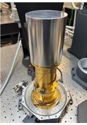
Step 5: Sorption cooler assembly installed on platform adapter.
