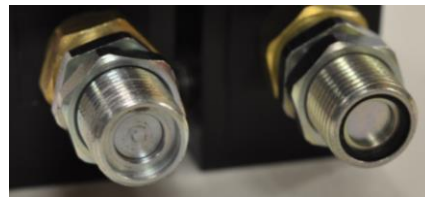
Fitting missing O-ring (left) and with proper O-ring (right)
