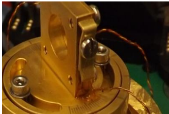
Wire lagged with VGE (clamp style)
