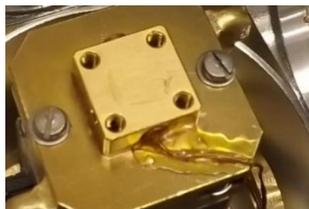
Wire lagged with VGE (plug style)
