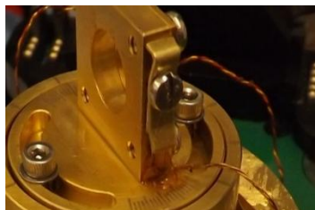
Wire lagged with VGE (clamp style)
