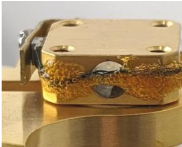
Step 3a: Thermometer clamped to the mounting surface
