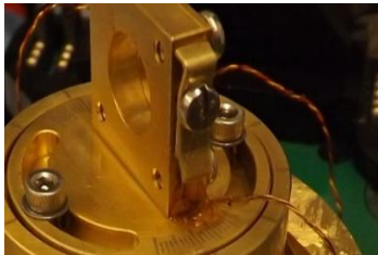
Wire lagged with VGE (clamp style)
