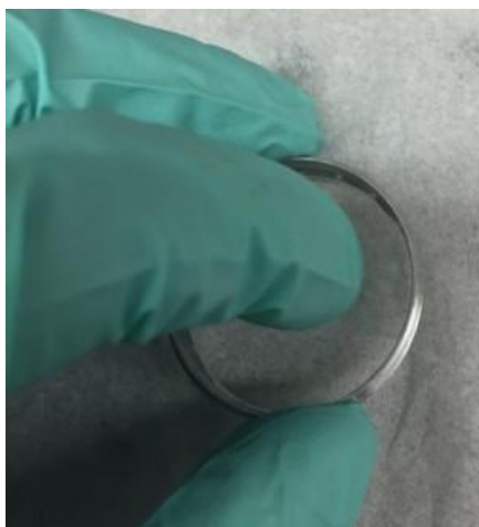
Pressing the window out of the tension ring
