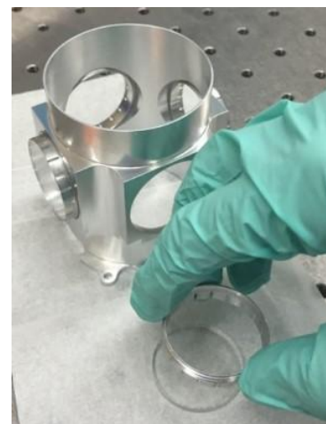
Pressing tension ring onto the window
