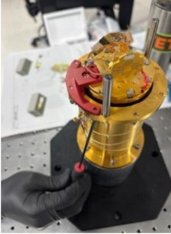
Step 4: Removing the pin shipping bracket.
