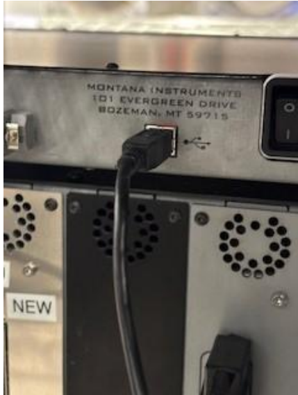
Step 14b: Connecting the Temperature Controller to the System Control Module (back of Temperature Controller).
