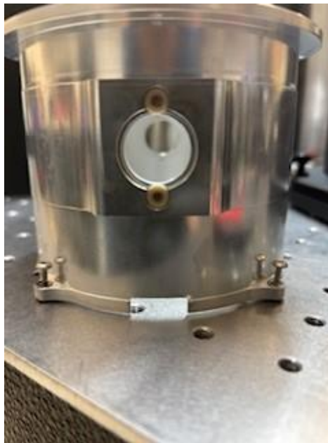
Installed radiation shield window.
