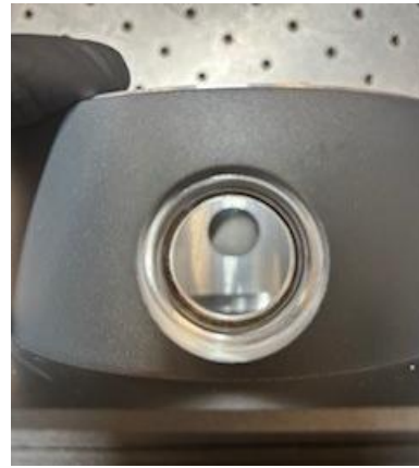
Step 3-4: Retaining ring and window removed, L-grease applied.
