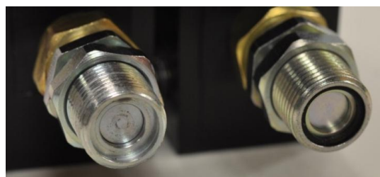
Left: Fitting missing O-ring Right: proper O-ring fitment
