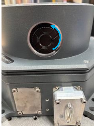
Window cover installed on standard vacuum housing.
