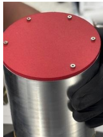
Step 10: Removing the sorption cooler shipping bracket.
