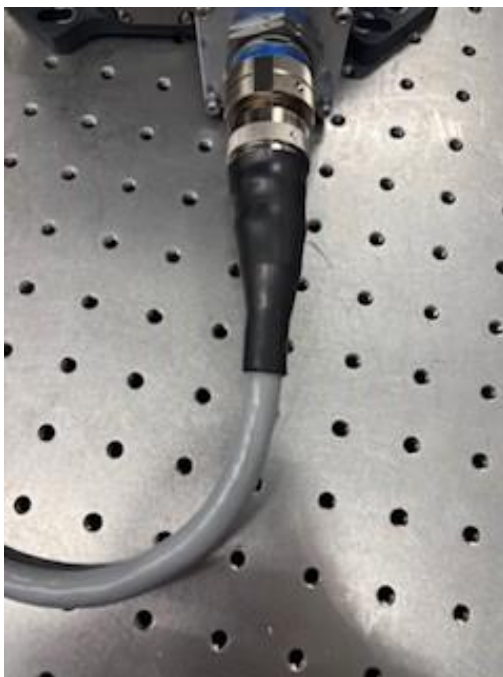
Step 14a: Connecting the side panel to the Temperature Controller.
