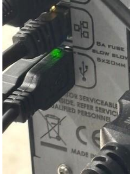
Step 14b: Connecting the Temperature Controller to the System Control Module (back of System Control Module).
