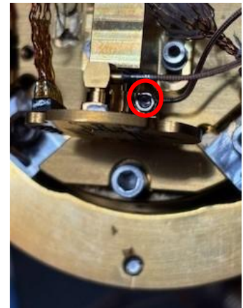
Step 5: Sample mount exchange, set screw circled in red.
