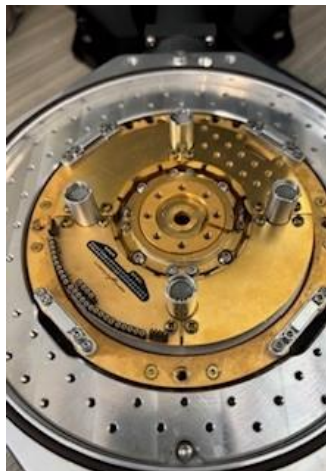
Step 1: Bare sample chamber (sample chamber surround plate installed).
