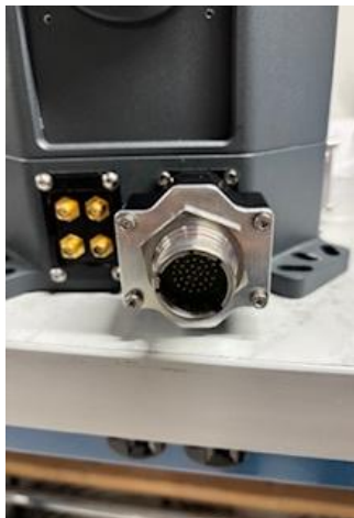
Step 2a: OneK-Optic operational side panel installed in position 4.
