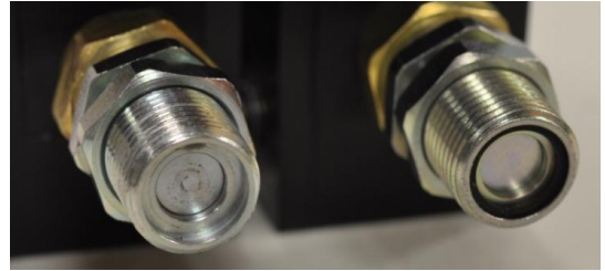
Left: Fitting missing O-ring Right: proper O-ring fitment
