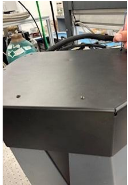
Reinstalling the top cover
