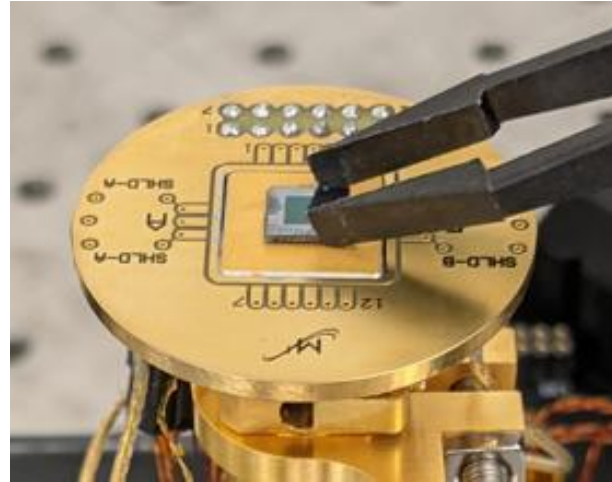
Step 3: Attaching new sample
