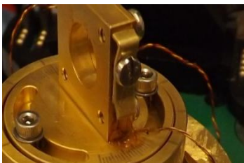
Wire lagged with VGE (clamp style)
