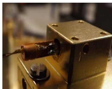
Thermometer installed in a plug
