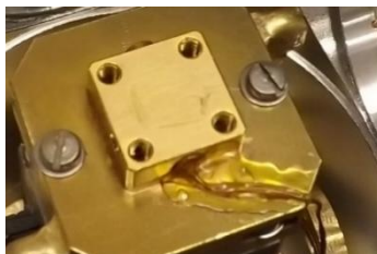
Wire lagged with VGE (plug style)
