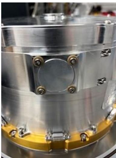
Step 1: Unscrew four M3 screws surrounding window or window blank
