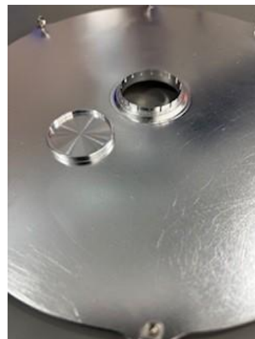
Window removed from tension ring
