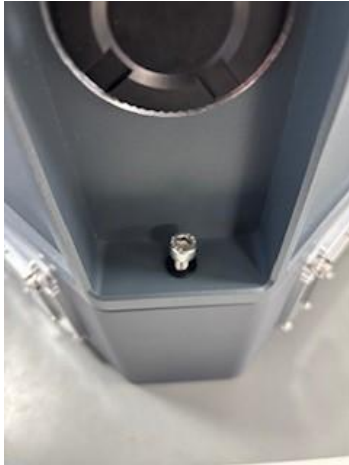
Step 1: Unbolting the vacuum housing from the lower sample chamber
